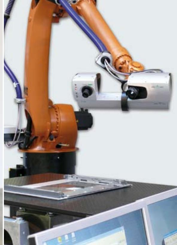
COMET5 is designed for applications in the most diverse areas of industry: Variable fields of view and a modular sensor concept allow for digitizing objects of a vast variety of sizes with highest precision.
